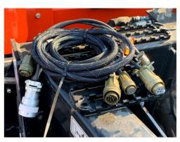
Machine Specific Kubota wiring harness makes installation simple and quick.
